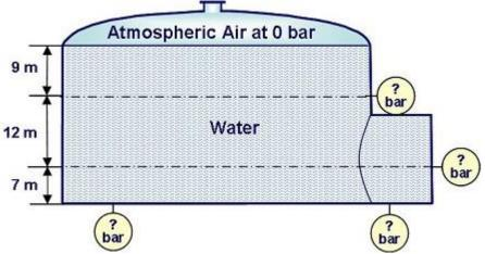
Indicate in [bar] the pressures in the tank.
