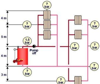
Pump off, we measure at the boiler a pressure of 3.5 [bar].
