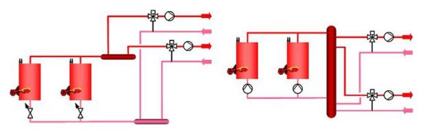
Variable flow boiler room ------ Constant flow boiler
