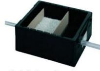
Neutralisation system using granules for condensate flows in gas boilers up to 70 l/h or 500 kW power approx.
