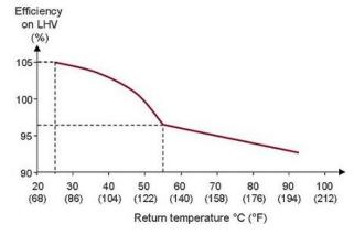
When the exterior temperature drops, how does condensing boiler efficiency evolve?
